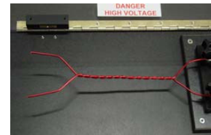
Twisted pair specimen in Dielectric Breakdown Test
